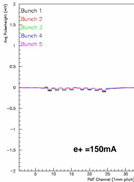
**Flat cable disconnected on DSP side (17May2005)**
