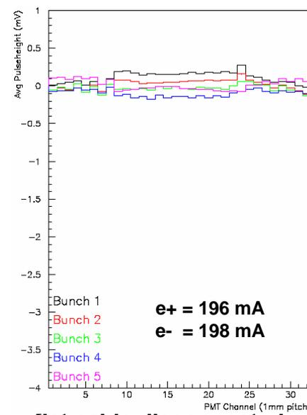
**flat cable disconnected on PMT side (24May2005)**
