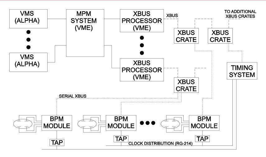
Key Feature: SERIAL-XBUS protocol provides 10K word/sec of transmission bandwidth all major processing must occur in DSPs, particularly when servicing many BPMs
