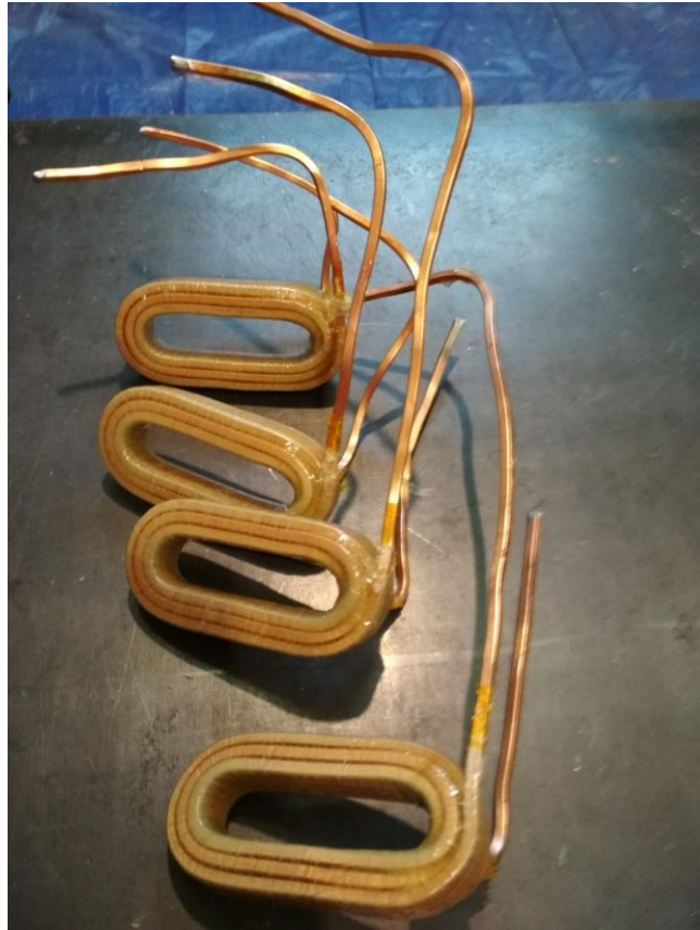
4 WATER QUADRUPOLE COILS: STATUS NOK Ground insulation OK Dimensional interference with the yoke. On progress
