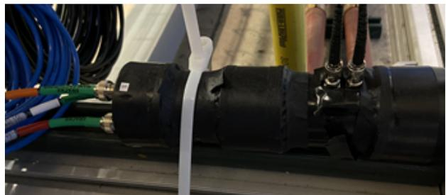
Figure 4 - PMT tie-wrapped to Girder
