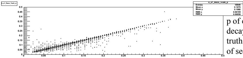
p of electron in reconstructed decay of second pi0 vs MC truth of electron from decay of second pi0
