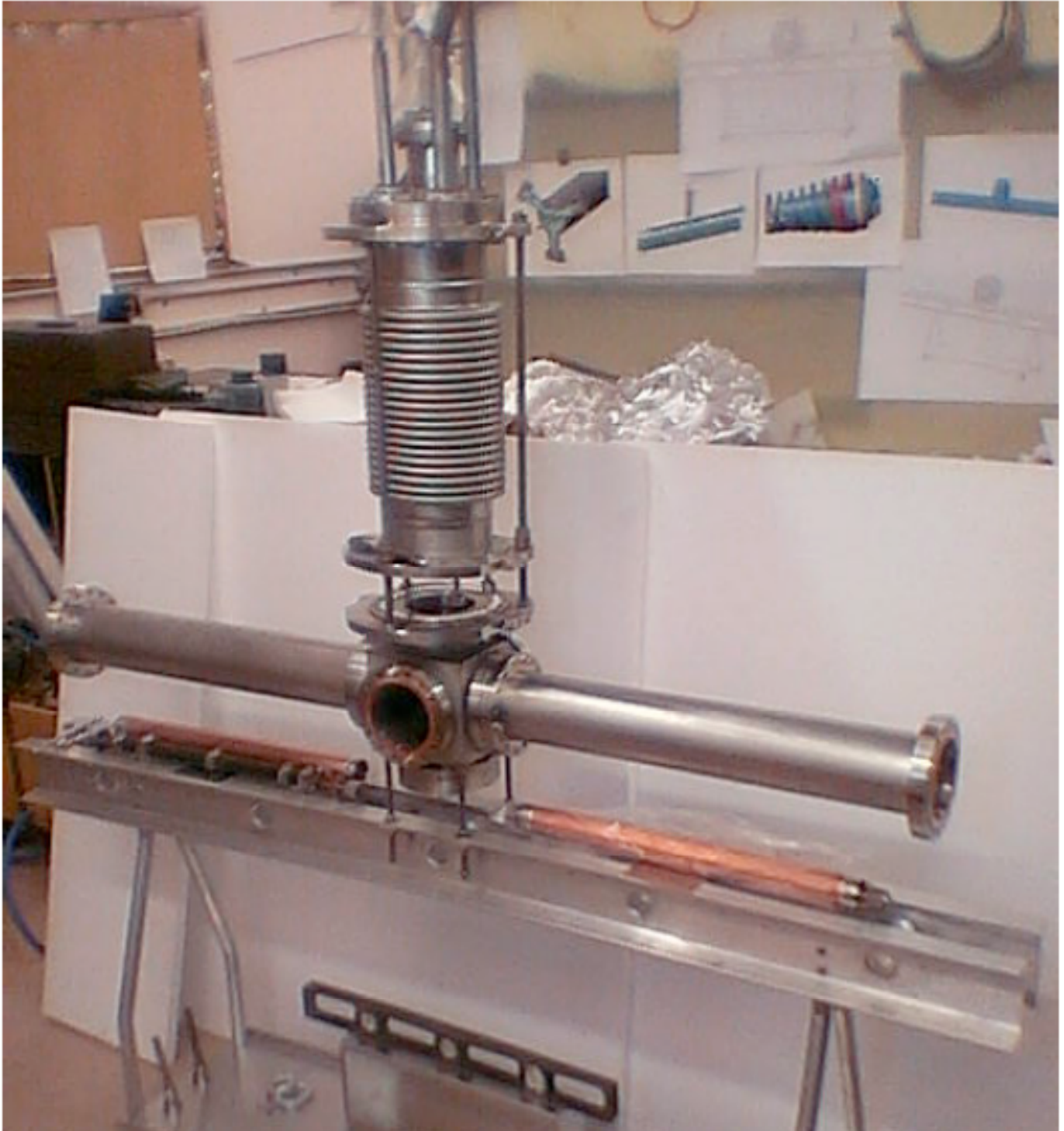
Fig. 6. 1m long model of undulator cryostat for testing with 40 cm model cores waiting for assembly
