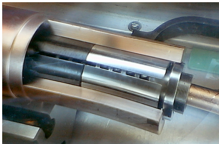
Fig. 3 Coil end of Figs. 1&2 during assembly of the model.
