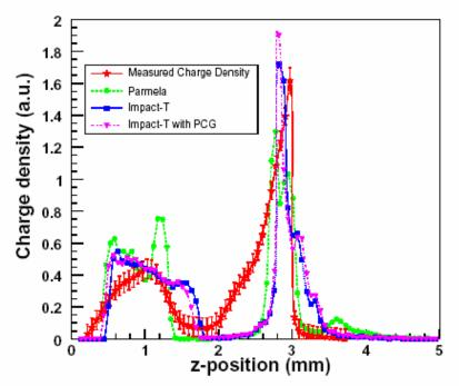
Figure 1: Reconstruction of the charge density associated to the 3.2 nC bunch produced at the Fermilab/NICADD photoinjector and comparison with three different beam tracking programs: "Parmela" from B. Young at Los Alamos, "Impact-T" from J. Qiang Lawrence Berkley lab. "Impact-T with PCG" is the NIU-version of Impact-T it uses a wavelet-based space-charge algorithm; see Reference [B. Terzic, *et al., Phys. Rev. ST Accel. Beams* **10**, 034201 (2007)].
