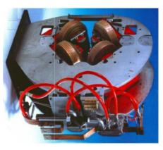
Energy Current Magnetic Length Magnet Bore Diameter Conductor Yoke: Magnet Weight Water Circuits per Magnet Coolant Hole Diam Conductor Size Ampere-Turns per Pole Field Quality Gradient 320 A 12800 75 mm 20 T/m 2 GeV 8.6 - 5.4 KW 470 - 230 mm < 10<sup>-3</sup> OFHC copper 9 x 6.8 mm<sup>2</sup> low carbon steel 1400 – 840 Kg Laminated Yoke -4.6 mm
