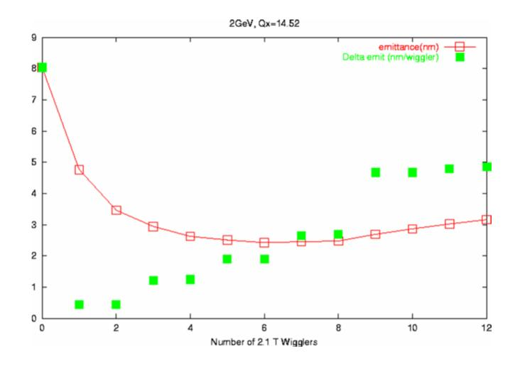
Wigglers deployed in lattice where  $\eta = \eta' = 0$   $\epsilon_{min} \sim 2.5 \text{nm}$  (6 wigglers)
