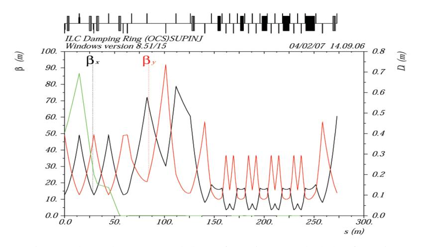
Six quadrupoles to match beta functions and alpha functions between arc and injection section.
