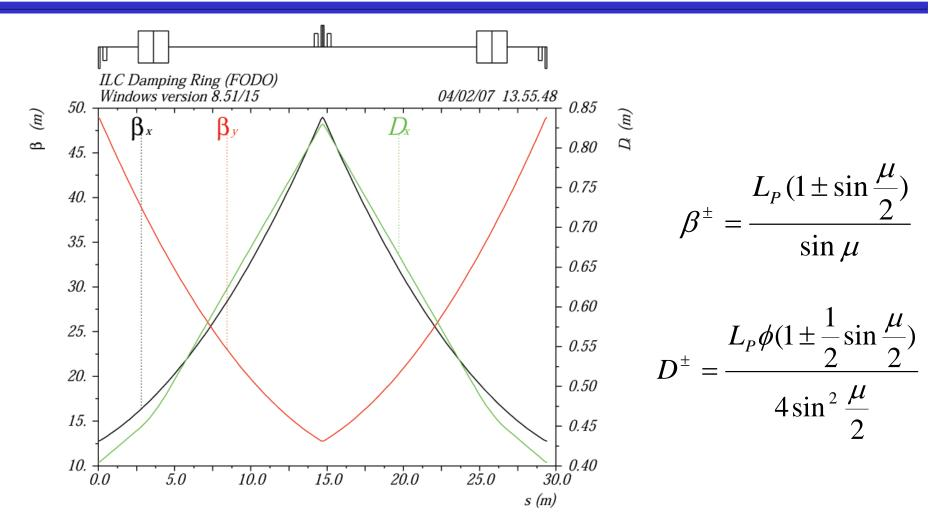
The 72/72 degree modified FODO arc cell is chosen. The cell length is 29.4 m. Adjust the drift length to get suitable betas and dispersion functions.
