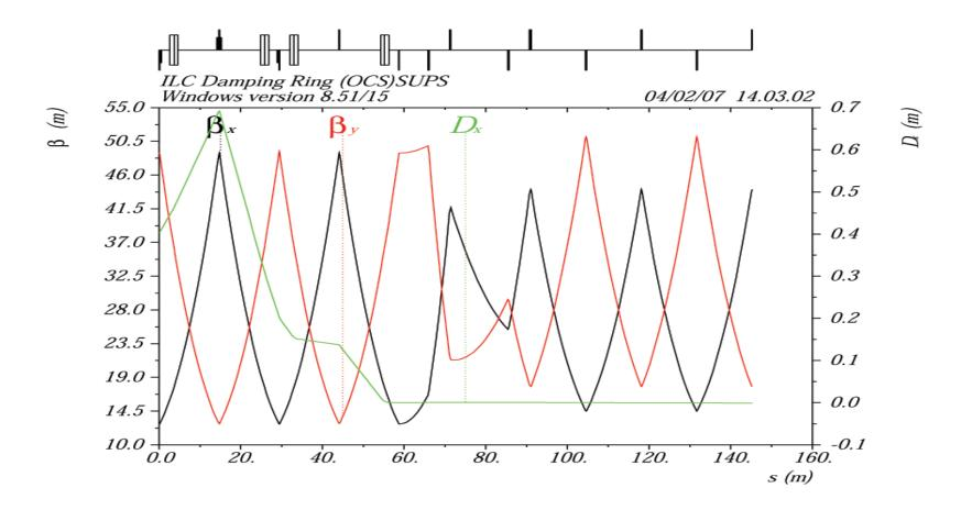
Four quadrupoles to match beta functions between arc and the extraction section.
