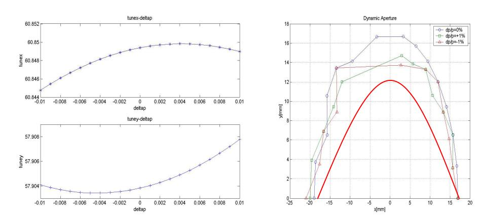
The chromaticity corrected to (0.15,0.15). The tune variation with momentum spread  $\pm 1\%$ ; the dynamic aperture with momentum spread up to  $\pm 1\%$  (with RF cavity, no errors).
