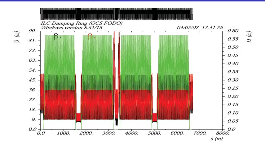
Adjusted the quadrupole strength in the match sections. There are 184 arc cells in all, maintain the circumference of 6695.057 m.
