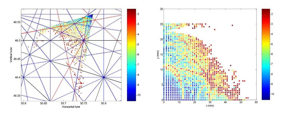
FMA analysis for on momentum particles: (Left) footprint; (Right) Dynamic aperture with FMA.
