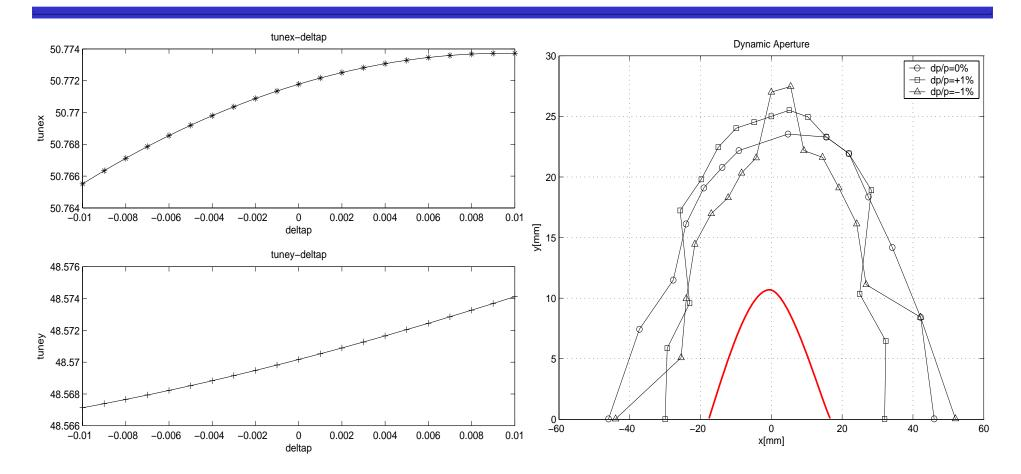
The chromaticity corrected to (0.3,0.31). The tune variation with momentum spread  $\pm 1\%$ ; the dynamic aperture with momentum spread up to  $\pm 1\%$  (with RF cavity, no errors).
