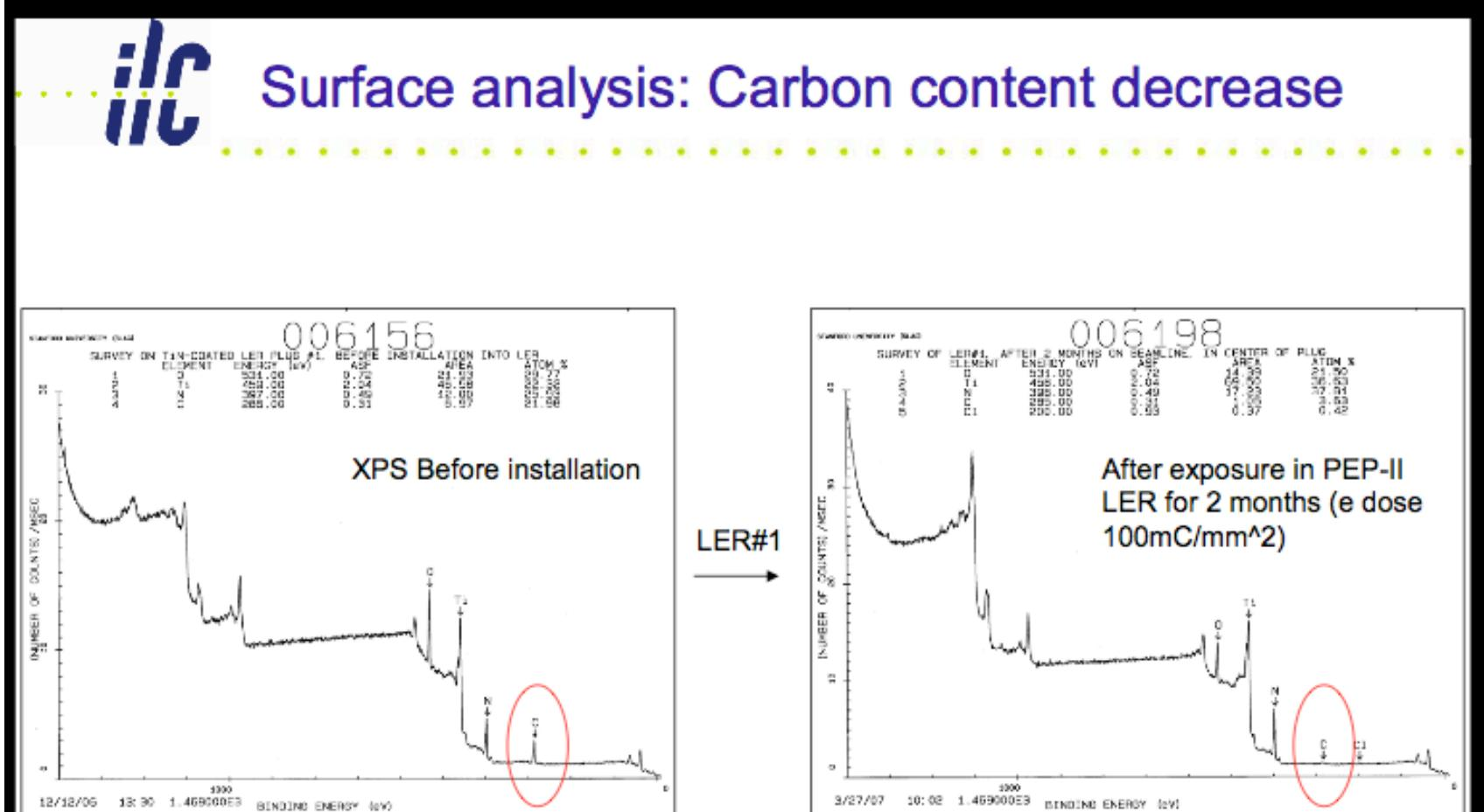
Different from electron conditioning in laboratory setup where carbon crystals grows!
