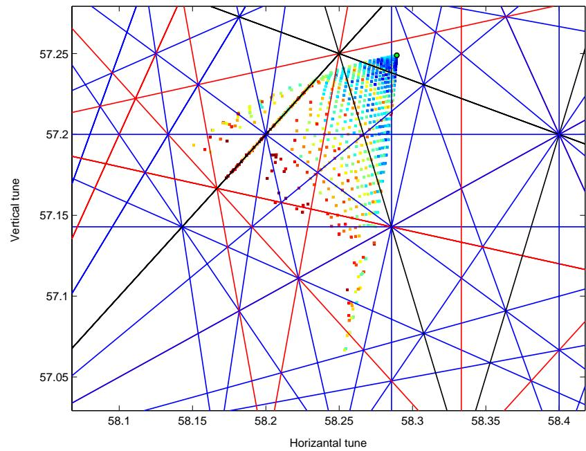
FMA is used to optimize the lattice and the DA. The optimized result for  $2 \times 10^{-4}$  momentum compaction mode
