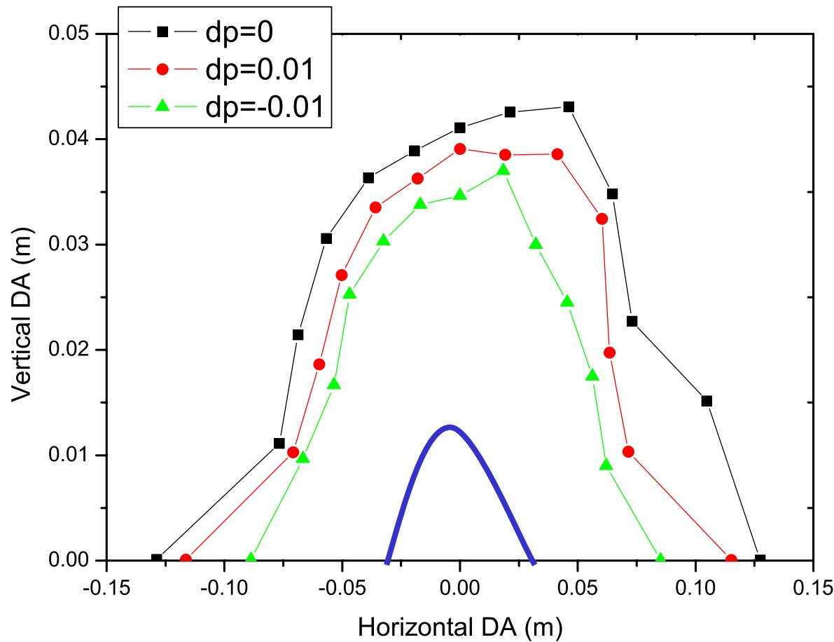
The blue line is **three times injected positron bunch size**.
