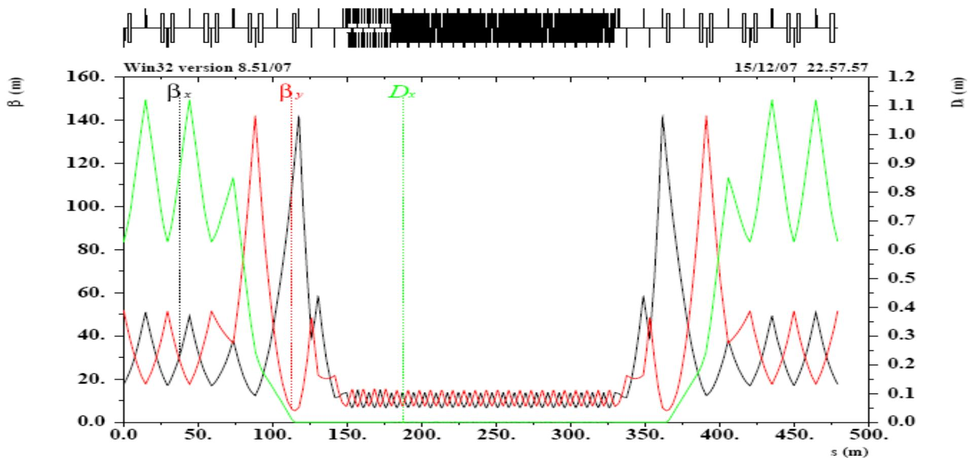
Tune the quadrupole's strength in the dispersion suppressor for the **60 degree case**, to make sure dispersion is free at exit, and dipole strength not changed (Geometry is the same).
