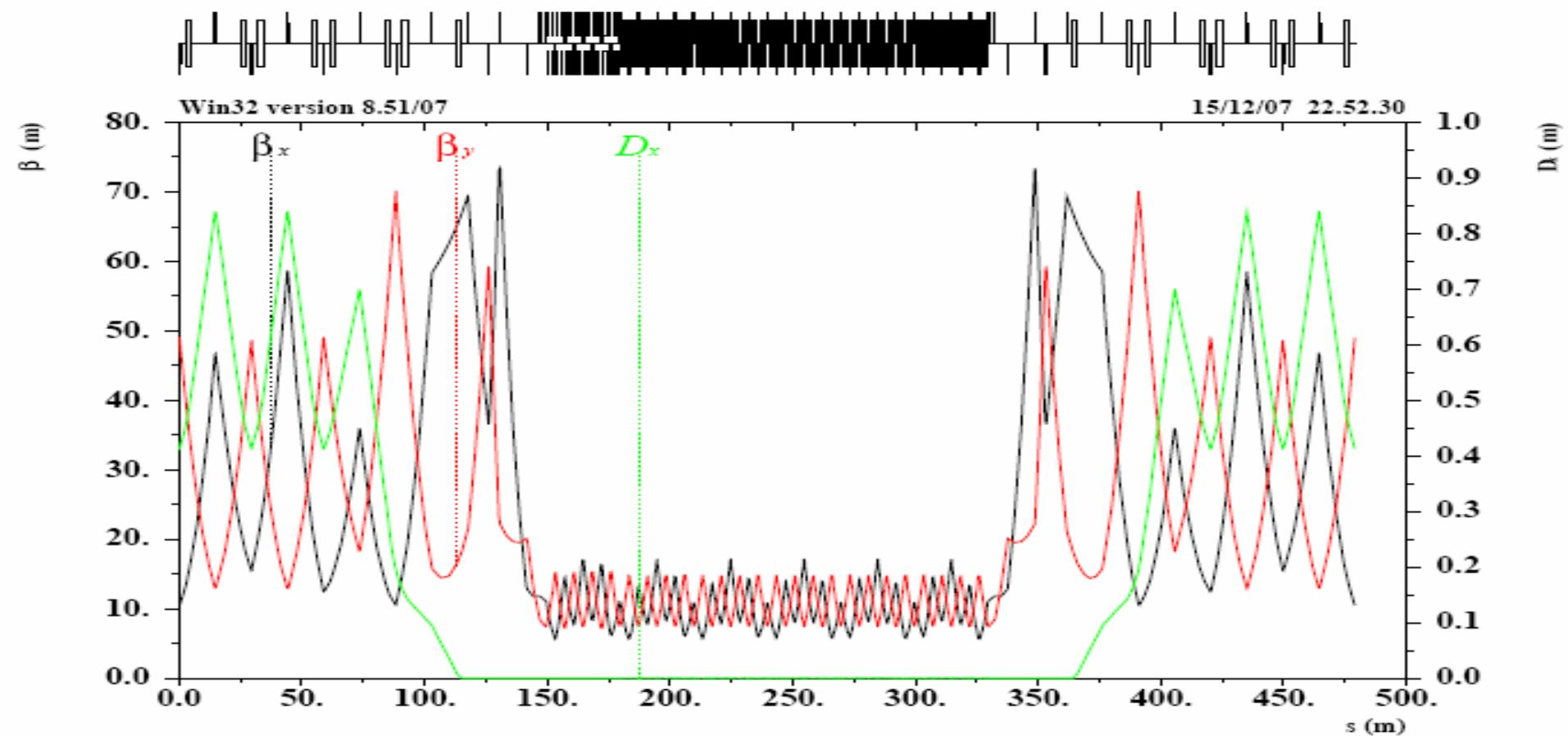
Tune the quadrupole's strength in the dispersion suppressor for the **72 degree case**, to make sure dispersion is free at exit, and dipole strength not changed (Geometry is the same).
