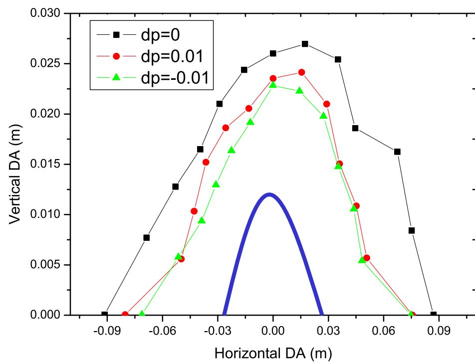
$4 \times 10^{-4}$  momentum compaction mode, on momentum particles, without errors; Left: OCS8, Right: FODO-4b
