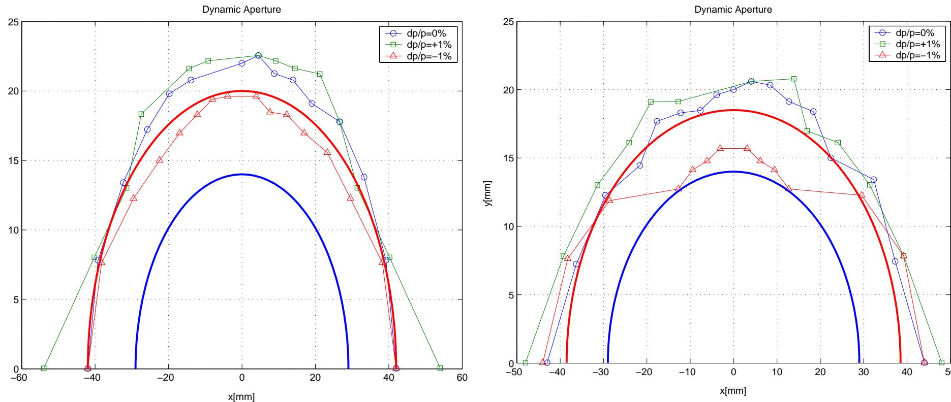
Left: no errors; Right: with high order magnets errors.
