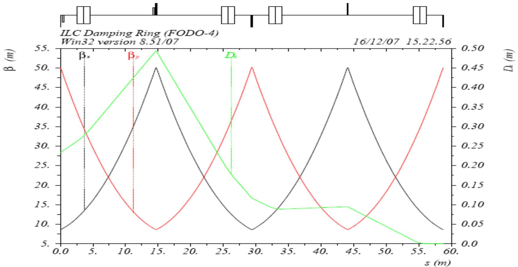
Select the **90 degree case** as the baseline, the bending angle in the dispersion suppressor is set to be half of the bending angle in the normal arc cell, so that zero dispersion at exit is got naturally for 90 degree case.
