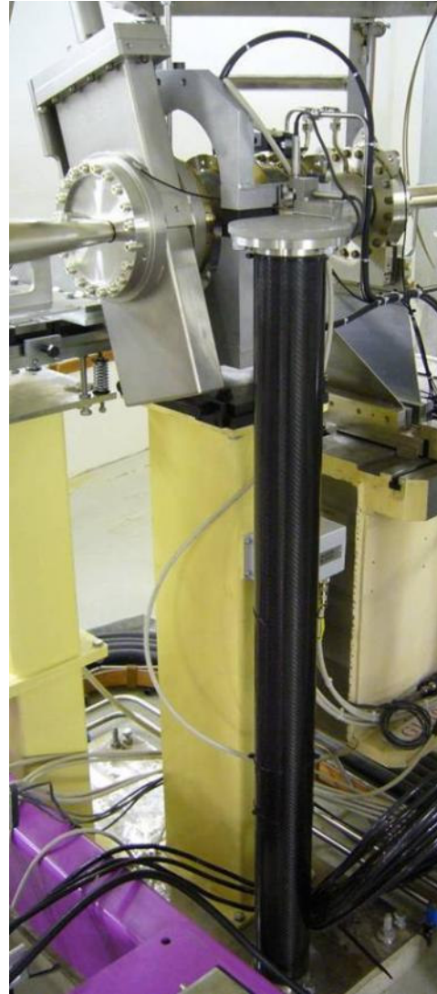
Reference pillar supporting linear encoders
