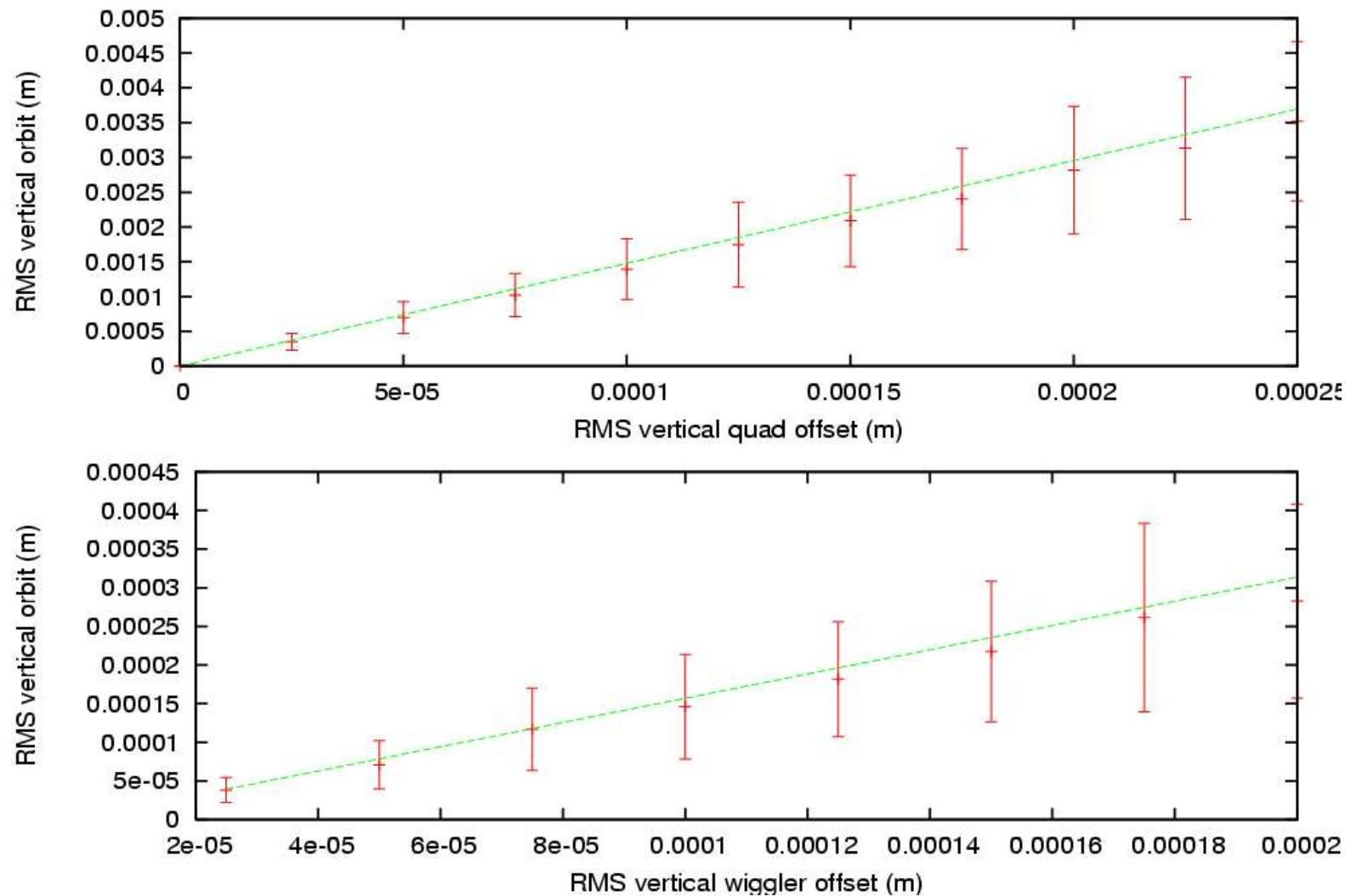
Phase correction corrects phase, however, nominal quad strength errors (RMS=.005) seem too strong. Plot uses (RMS= .001).
