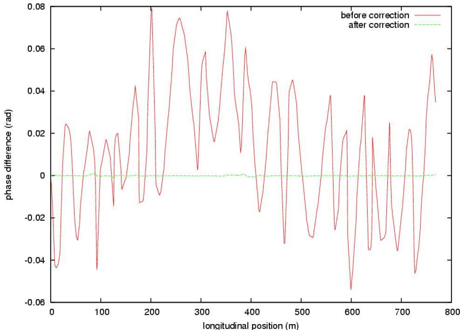
Correcting phase with only quad strength errors does not significantly improve emittance.
