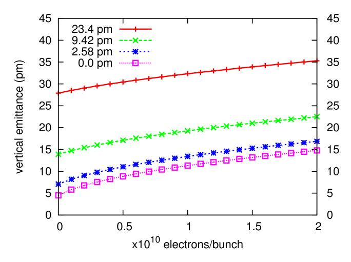
This plot shows the equilibrium vertical emittance as a function of particles per bunch. The 0.0 pm data represents vertical emittance assuming a perfectly flat lattice, but with .25% emittance coupling.
