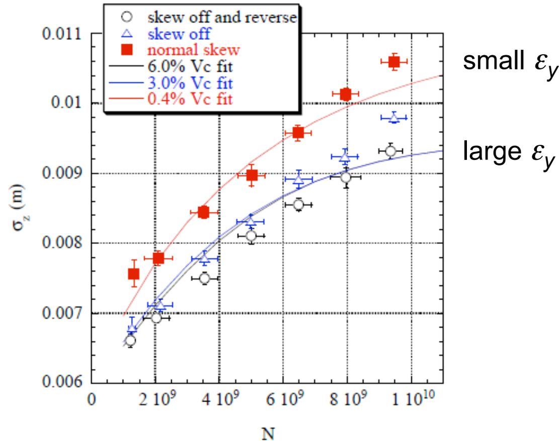
Difference between calculation and measurement may come from non-inductive components of impedance.
