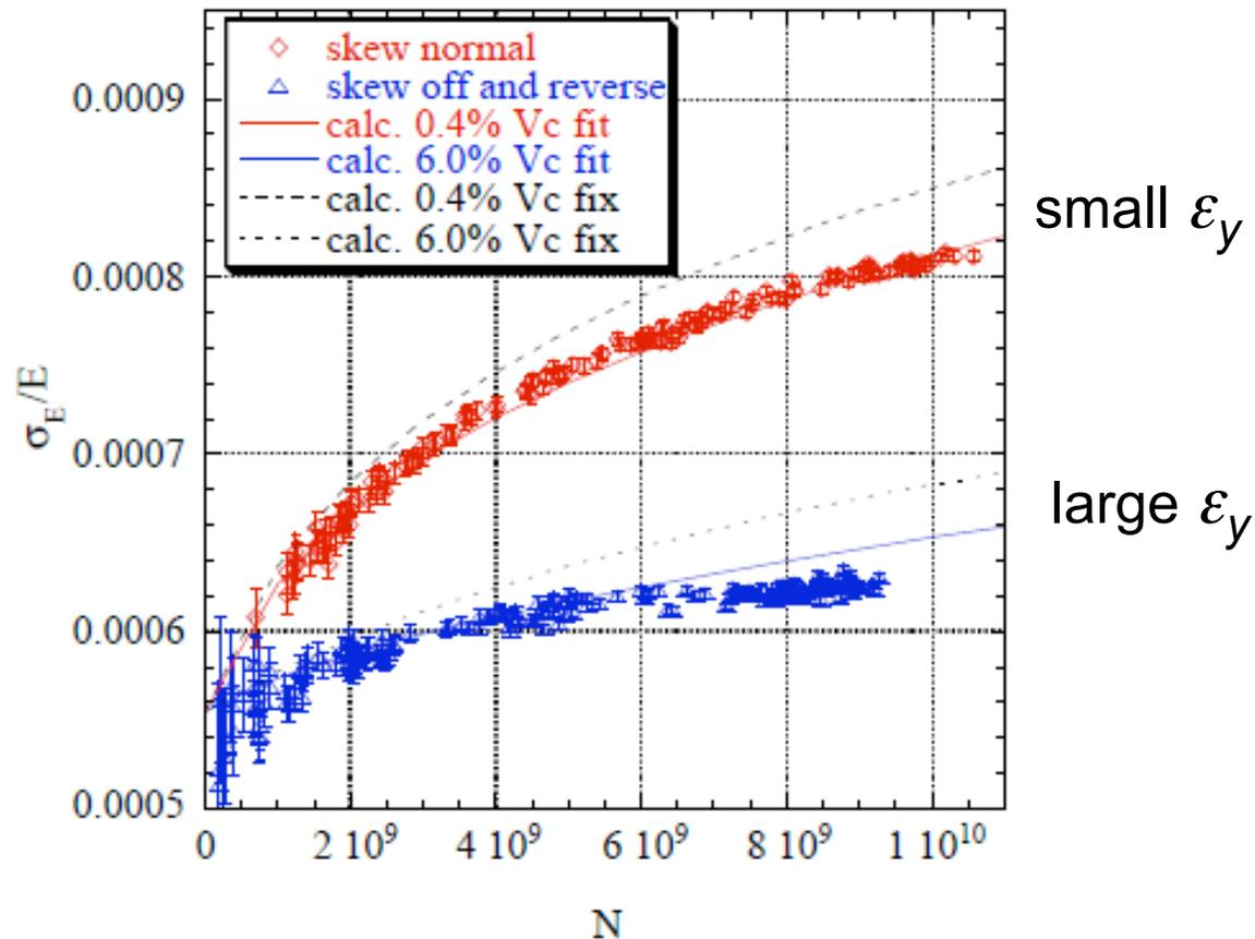
Calculation with fitted  $V_c$  (which was fitted to reproduce measured bunch length) agree with measured momentum spread data much better than fixed  $V_c$ .
