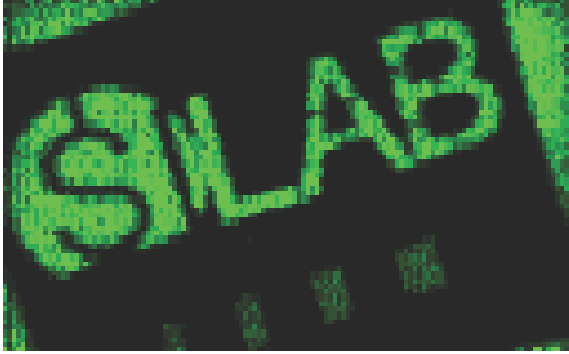
Figure 9. Radiogram of a 10\ \mu\text{m} thick tungsten logo irradiated by ^{55}\text{Fe} taken with the ILC-DEPFET system.
